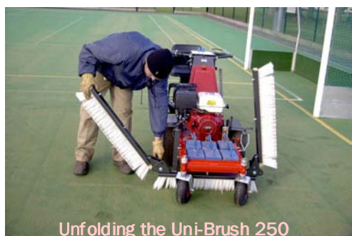
Sand removal brush for renovation
