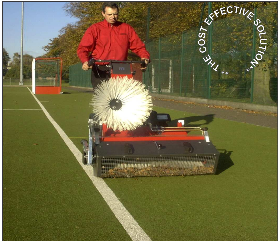
Simple separation of the surface filling from debris using the filter box
