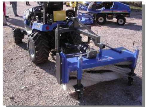
HFKM 1250 Pto drive with no collector with manual angling and compact linkage frame
