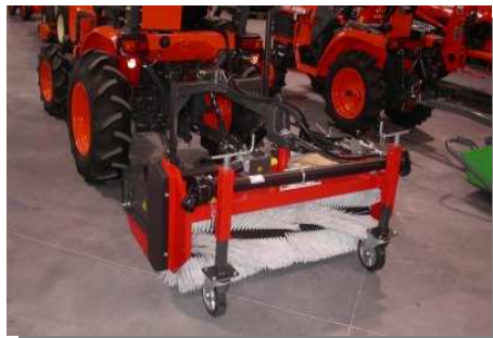
HFKM 1250 Pto drive with hydraulic empty collector and hydraulic side gully brush
