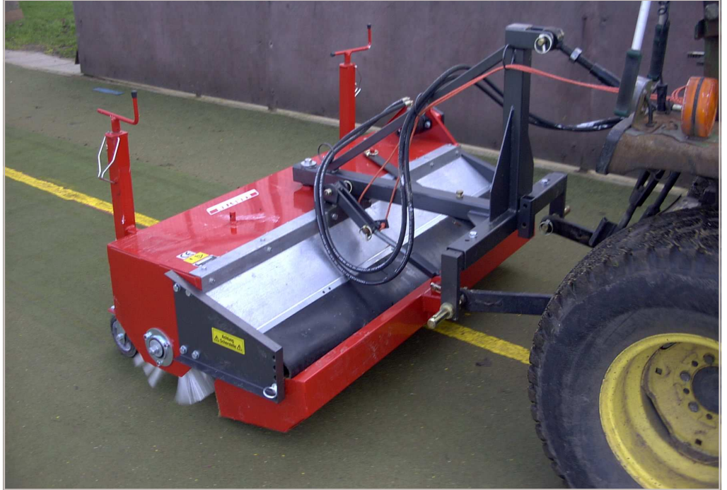
HFKM 1500 with hydraulic drive, manual collector and manual angling
