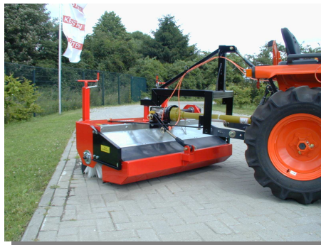
HFKM 1500 with Pto drive manual collector and manual angling
