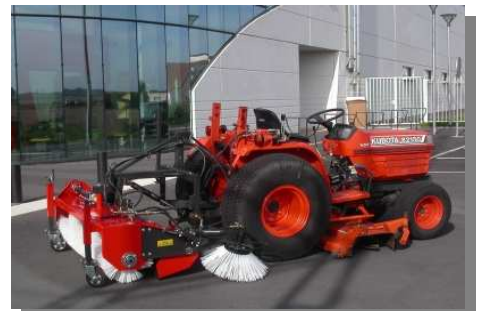
HFKM 1500 Pto drive, hydraulic empty collector and hydraulic side gully brush
