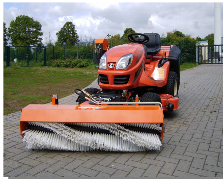
Front sweeper available with collector and side gully brush
