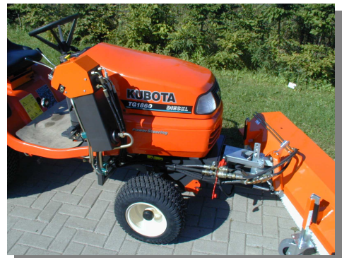
FKDR/HydrDL includes hydraulic lift and lower and angling.
