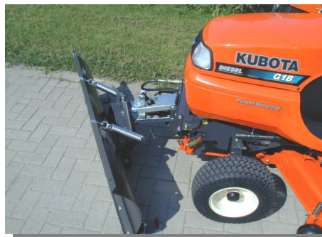
Snow Blade on FKDR available with manual lift and lower or hydraulic
